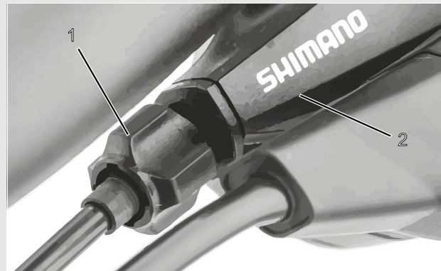
Figure 56: Adjusting sleeve (1) for the single-cable, cable-operated gear shift with shifter housing (2), example
