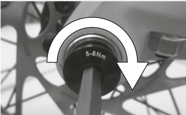
Figure 14: Tightening the securing screw
