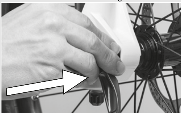
Figure 24: Pushing the quick release in
