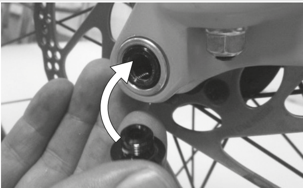
Figure 13: Pushing the quick release lever into the axle
