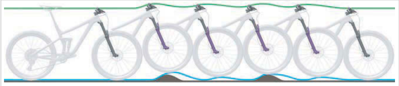
Figure 199: Suspension fork rebounding too quickly
