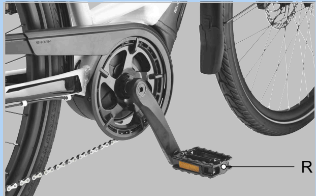
Figure 89: R-pedal in the right-hand crank arm
