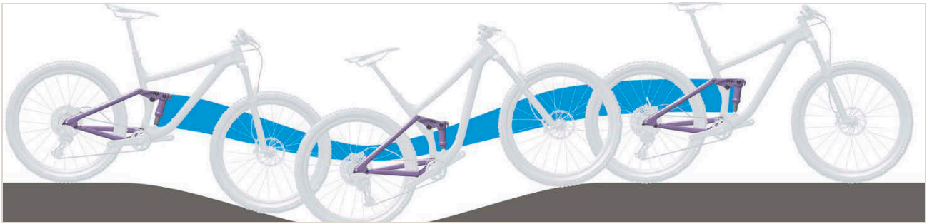
Figure 209: Excessively soft suspension in the rear frame damper on hilly terrain
