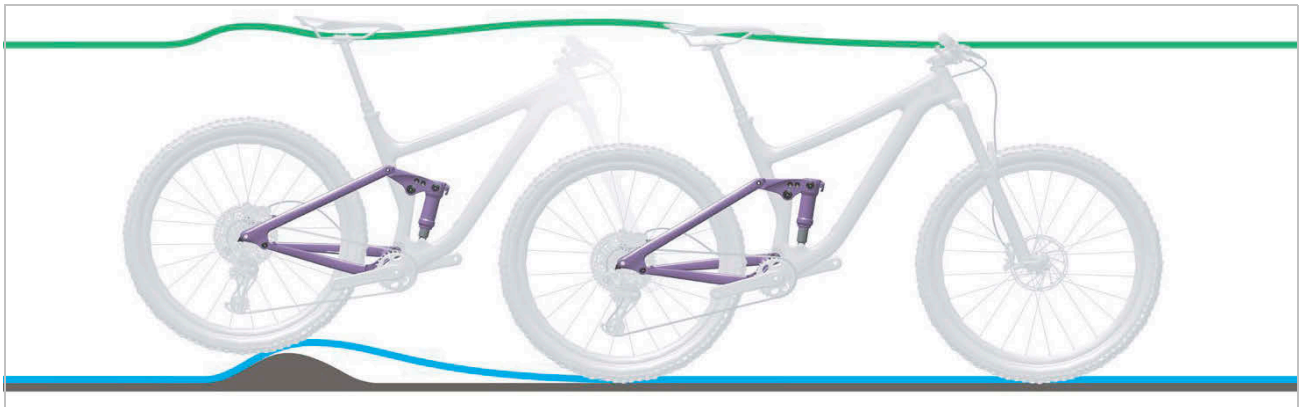
Figure 211: Excessively hard damping in the rear frame damper on bumps
