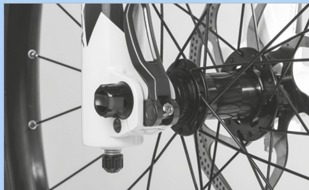
Figure 194: Adjusting the quick release clamping force
