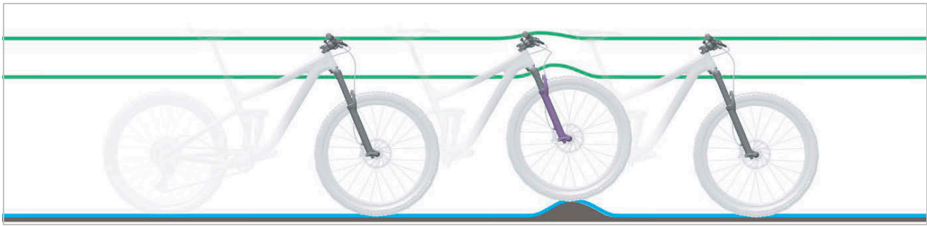
Figure 20: Optimum suspension fork ride performance over bumps
