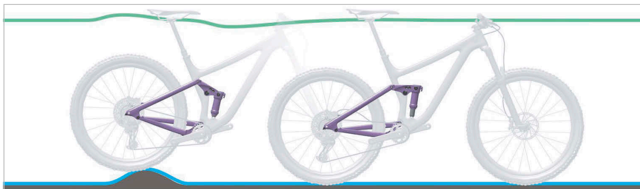
Figure 127: Optimum rear frame damper ride performance over bumps
