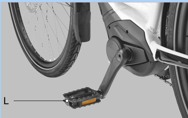
Figure 88: L-pedal in the left-hand crank arm
