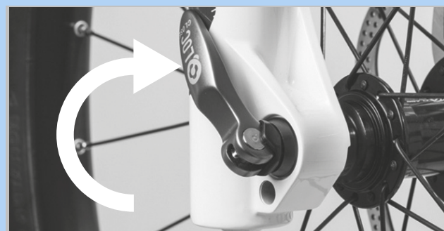
Figure 86: Closing the quick release
