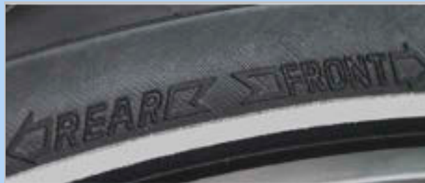
Figure 72: Rotation direction arrow on MTB tyres
